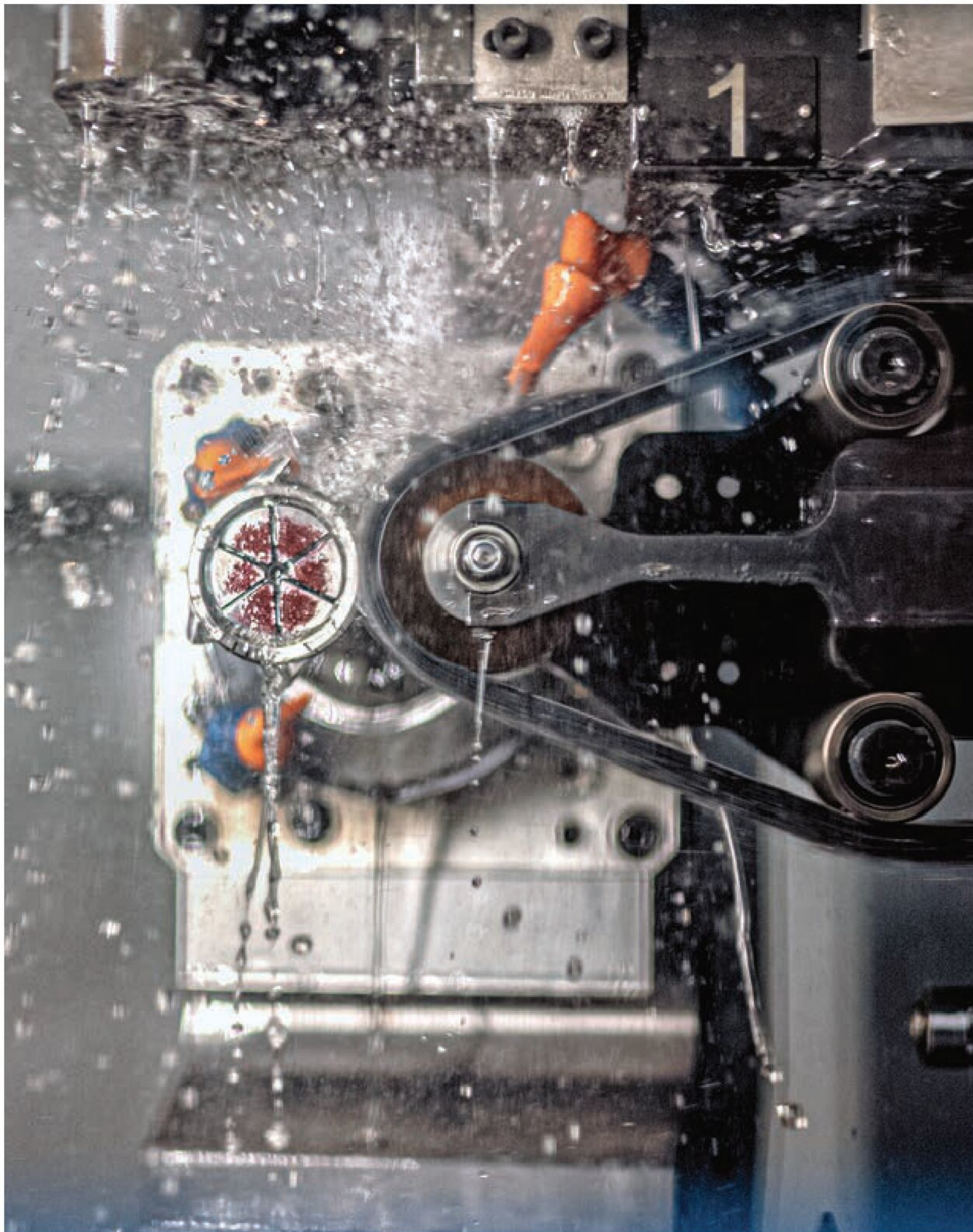
Machinery polishes a watch case
